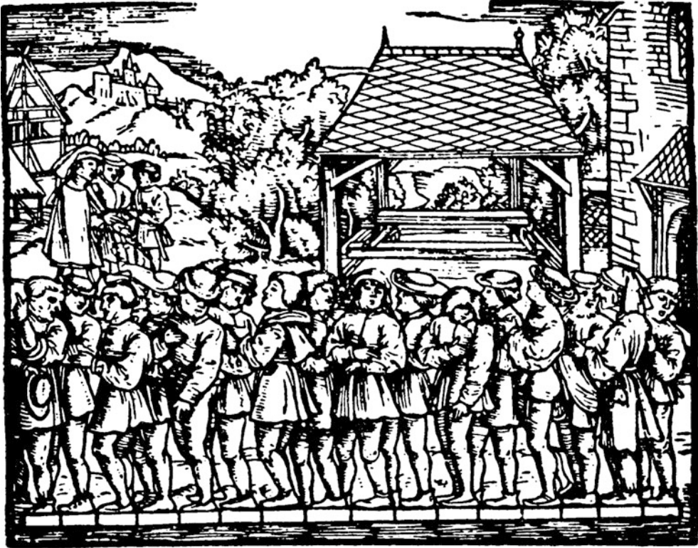
Determination of mean foot length Woodcut from Jacob Köbel's "Geometrei" published 1575 in Frankfurt
